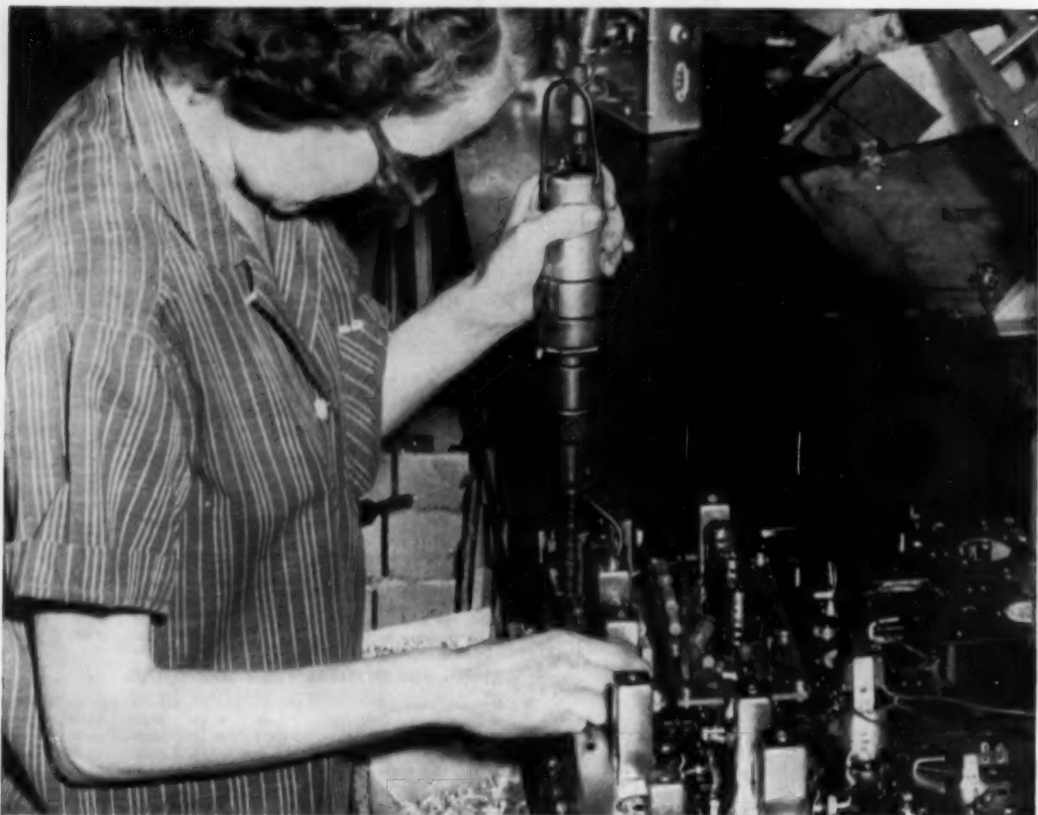
Operator fastens printed circuit assembly to color television chassis—with Keller Tool screw driver.
